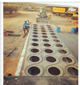
Trolley type design can load 42 asphalt drums in one, it is perfect choice for huge quantity production.
